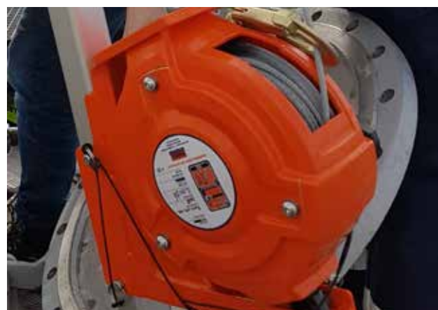
Man Riding Winches type MRW33 & MRW15 with modular quick-mount brackets on tripod on tripod leg
