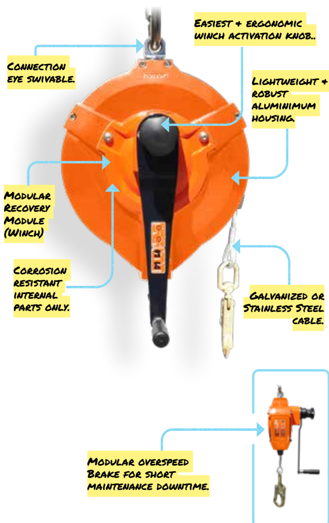
Man Riding Winch (type MRW33) on tripod with Fall Arrest Recovery Block type FAB33R for safe confined entry & rescue
